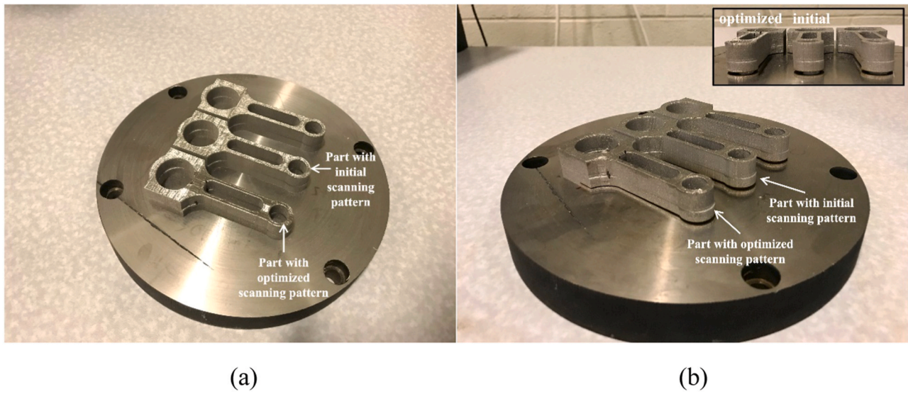
Fig. 12. As-built connecting rods with initial and optimized scanning pattern: (a) before sectioning; (b) after sectioning.
